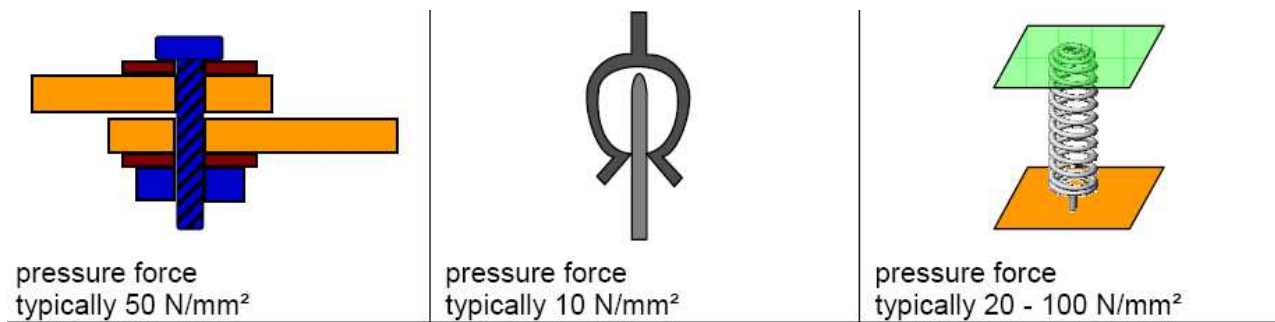
Figure 2.5.7 Comparison of contact pressures of detachable electrical connections (from left to right: screw, plug-in, spring contact)
