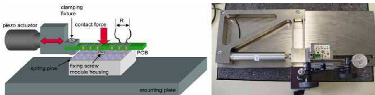
Figure 2.7.5 Schematic drawing and photograph of the micro-vibration test, exemplary test of MiniSKiiP springs
