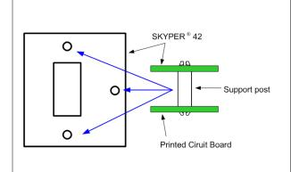
The connection between driver core and adaptor board should be mechanical reinforced by using support posts. The posts have to be spaced between driver core and adaptor board.
