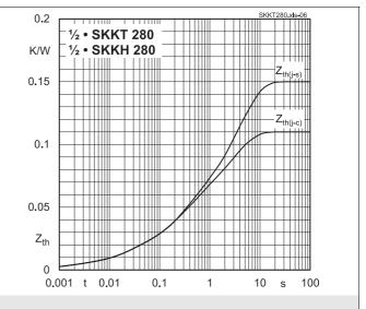
Fig. 6: Transient thermal impedance vs. time
