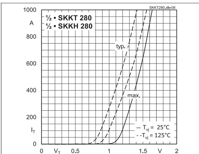
Fig. 7: On-state characteristics
