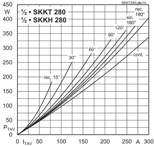
Fig. 1L: Power dissipation per thyristor vs. on-state current
