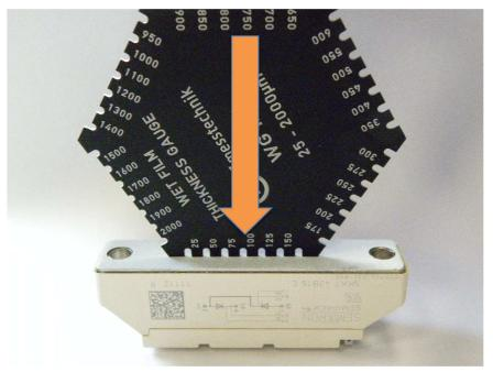
Visually inspect the marks. The result is always between the highest visible mark and the next non-visible one. In the left orange circle, there is s slight mark still visible; not in the right one. Therefore the measurement result is in between 0,050 - 0,075mm.
